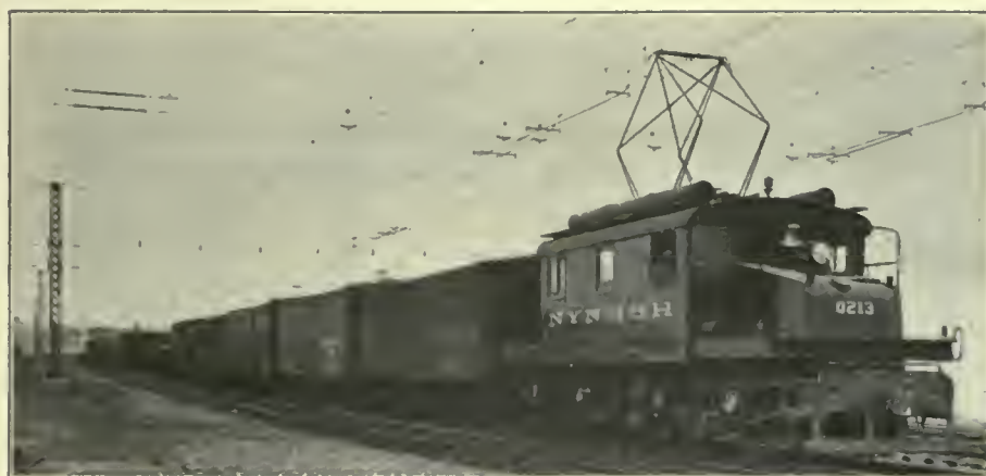
FIG. 539. ELECTRIC LOCOMOTIVES. Switching Locomotive for 11,000-Volt Single-Phase Overhead Contact Operation, New York, New Haven & Hartford Railroad.
